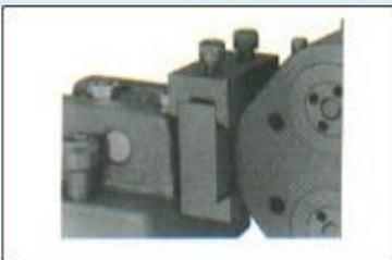
The dovetail design of the connection between the head and the adapter makes it possible to easily remove the head from the machine for changing or adjusting rolls, or for convenience in making adjustments, without removing the adapter from the cross slide. This feature combined with an adjustable and positive locating stop, assures that the head will always be reassembled in the adapter in the same relative position to the work.
