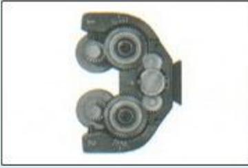
Roll "wind-up." caused by one roll rotating counter to the direction of attachment advance as the rolls move into the work. is automatically compensated for, by an advance compensating device within the head without placing any undue strain on the gear train. The Advance Compensator insures perfect synchronization of the thread rolls during rolling operation.
